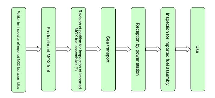
\* "Revision of petition for inspection of imported MOX fuel assemblies" means that we will submit a "Material Concerning Test Results" and "Explanation of Quality Assurance" after fuel production is complete as part of the imported MOX fuel assembly inspection petition, as based on Article 78-2 of the Electric Utility Law enforcement regulations.
