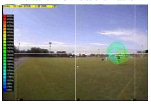
If there are sounds of different frequencies from the same direction, measurements from the earlier sound camera are shown overlapping as on the right. This made it impossible to determine the frequency of the sound source objects in front and back.
