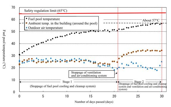
Figure 1. Results of fuel pool water temperature measurement (September 6 – October 6, 2011)
