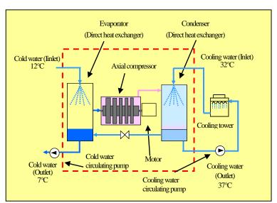
Water acting as refrigerant circulates from the evaporator to the axial compressor, then to the condenser and back to the evaporator, while being mixed with cooling water and cold water.
