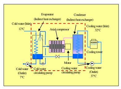
Water acting as refrigerant circulates from the evaporator to the axial compressor, then to the condenser and back to the evaporator (the refrigerant for this section has been switched from fluorocarbon to water).
